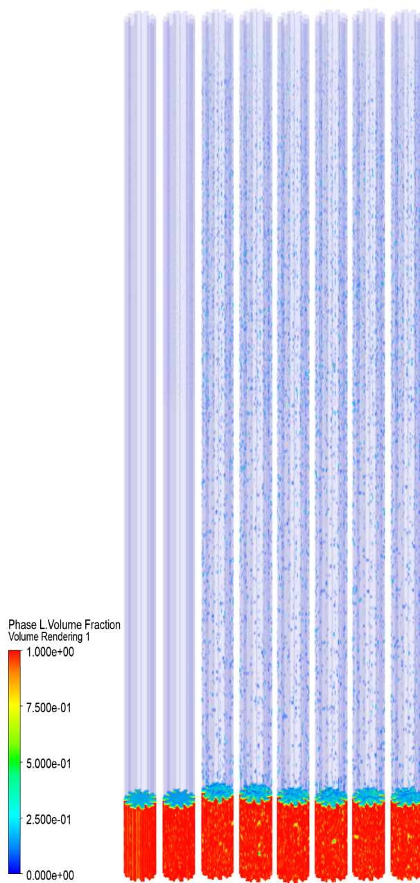
Figure 2. Evaporation and condensation contours of THP in 0.1-0.2-5-15-50-100-150 and 200 seconds, respectively
