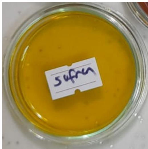
Figure 2. Photoanode layer dipped saffron dye.
